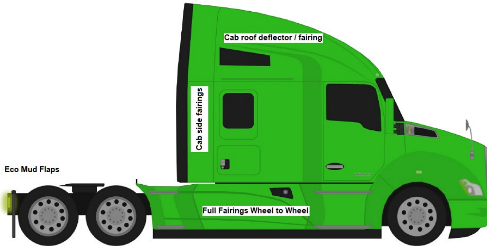
Image 4: Cab roof deflector/fairing, Cab side fairings, Full fairings wheel to wheel, Eco Mud Flaps
